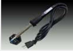
**XY-200PHG25:** 25Watt Plug and Play soldering iron. Heavy duty with grounded 3 wire, Includes pre-loaded tip. Maximum temperature range: 338°C/640°C—Choose from 44-240503 & 44-240517 replacement soldering tips.
